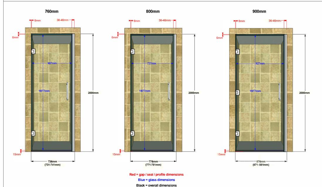
760 / 800mm door is supplied with 2 hinges 900mm door is supplied with 3 hinges Bespoke sizes available on request
